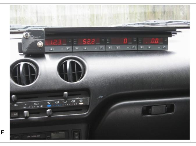
The electric Toyota instrumentation. From the left is the ignition switch and starter button for a generator, Voltmeters for the 12 and 48 Volt batteries, and ammeters for the motor and the generator.
